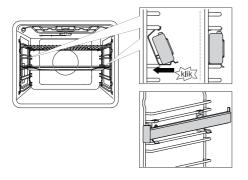
The click-on pull-out guide can be inserted into any space between two wire guides.
